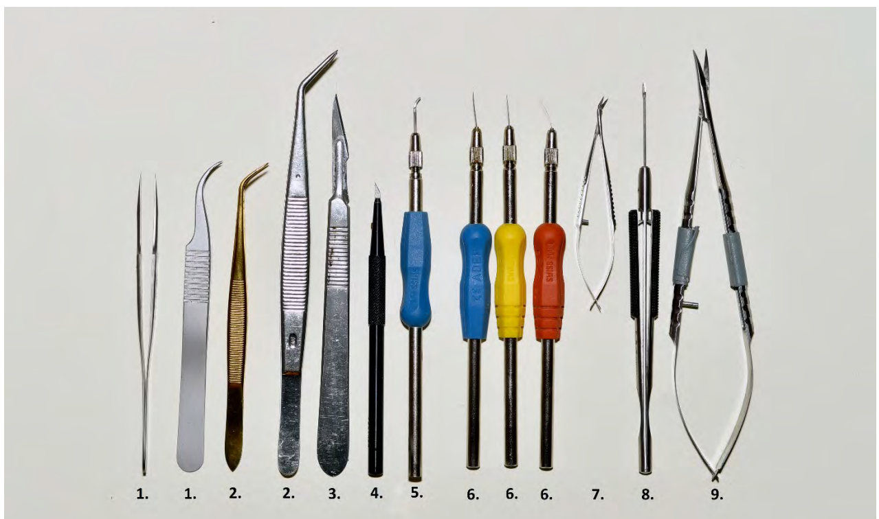
Fig. 1. Useful dissection tools. Straight and curved tweezers (1); different sized forceps (2); normal sized scalpel (3); micro scalpels (4); needle scalpels (5); three tungsten needles (0.3, 0.2 and 0.1 mm diameter sharpened tungsten wire) (6); small micro scissors (7); long vitrectomy scissors (8); and large curved scissors (9).
